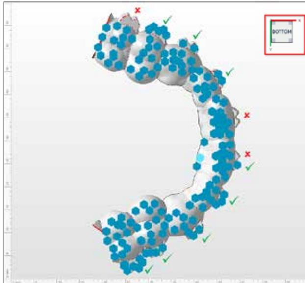
To set new bars, select the function »Create new bar« in the upper menu toolbar. Double-click on the point on the splint to be supported to create a new support bar (alternatively: left-click to set an anchor point, right-click on the anchor point and click on »Create bar«).
