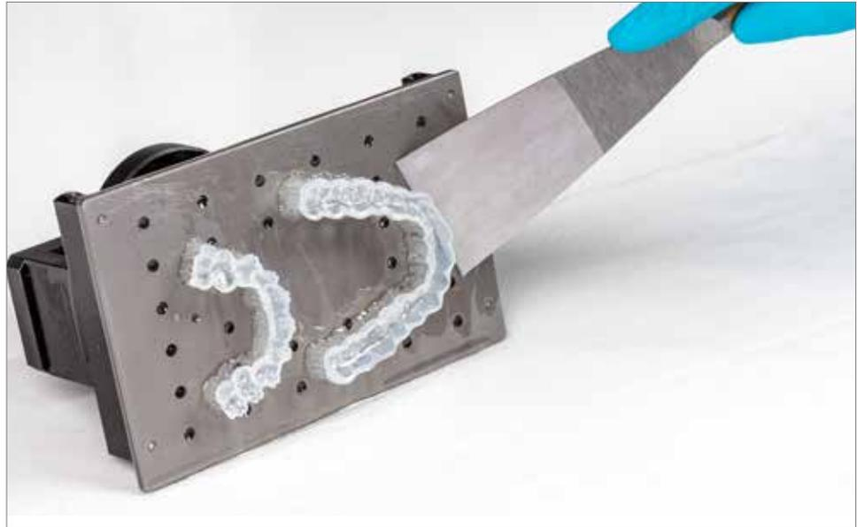
In the case of highly adhesive objects, carefully hit the handle of the spatula with a hammer to detach the baseplate of the printed object from the building plate. Always be careful not to damage the splints.
