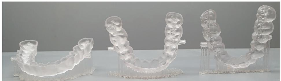
Aligning the splints in Netfabb, including support structures.
