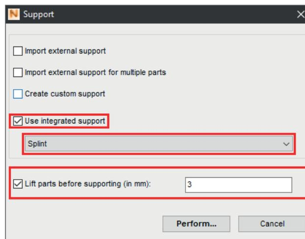
The program automatically calculates the optimal position of the supports and inserts it between the building plate and the splint. Please examine the object for incorrectly placed support structures. No support structures should be found on the inner surfaces relevant for the fit. If necessary, remove individual support structures using the editing feature.
