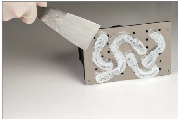
Figure 17: Loosening the printed objects from the build plate
