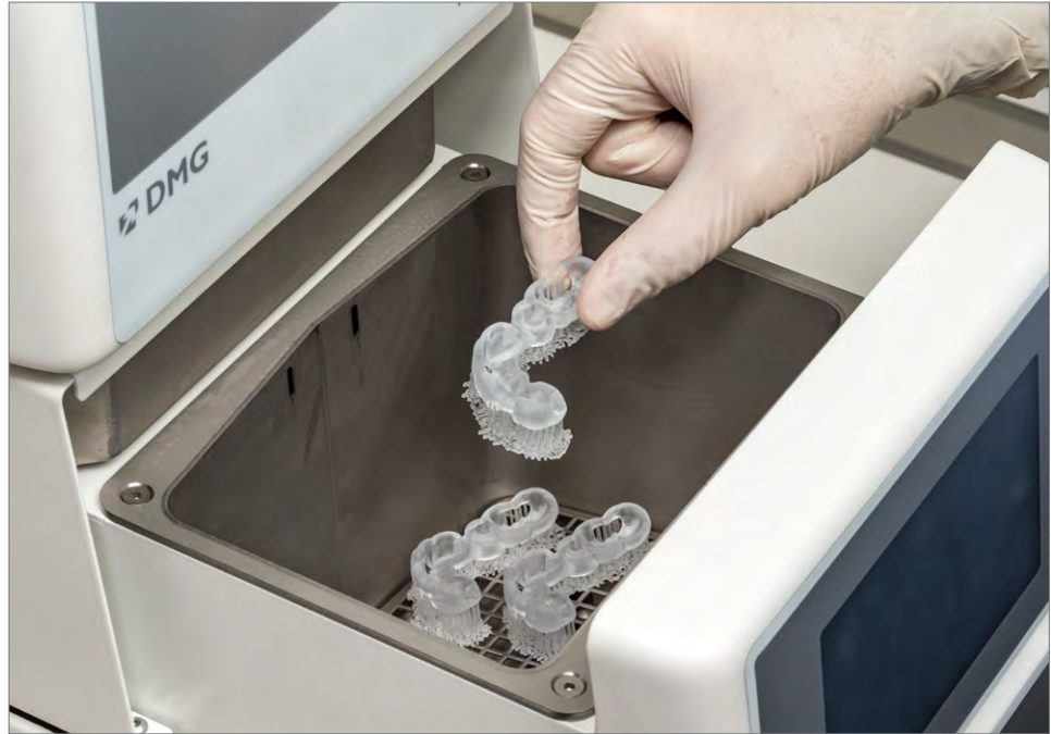
Figure 18: Drilling sleeve in the 3Dewash unit
